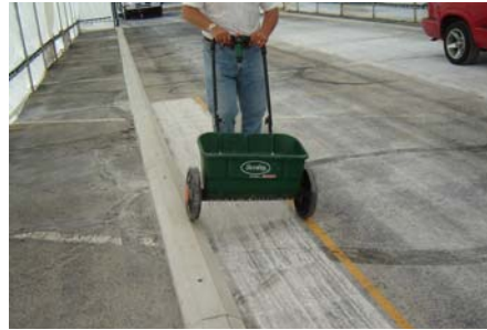
Spreading the dust simulant on the test track
